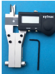
Place caliper jaws in holder slots
