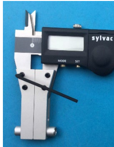
Fasten the 4 grub screws carefully
