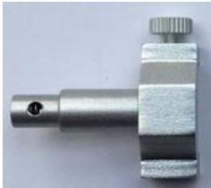
Caliper accuracy can be determined by using a calibration plate as reference on d2 and use of a pressure device FMS A40. Measurement accuracy to within  $\pm 0.01\text{mm}$  /  $0.0004''$  is then possible. When thread pitch diameter is measured at machine set up, if a solid gauge is used for inspection, then wear will be significantly less if the manufactured thread tolerance is kept away from the upper and lower tolerance limit. A thread with a good fit is never too loose or too tight.
