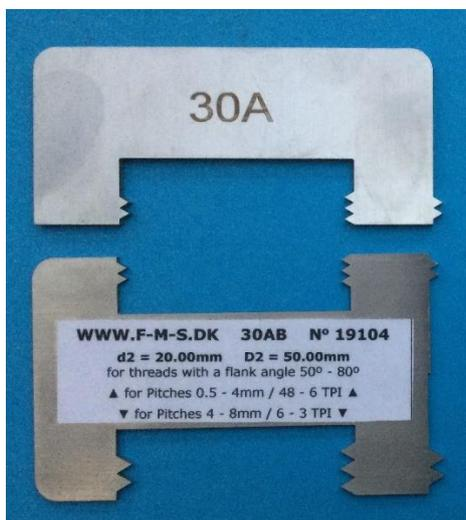
Calibration plates starting with 30 are for thread inserts starting with 21, 22, 23, 24 and 25.
