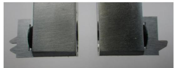
Buttress 3mm pitch internal
