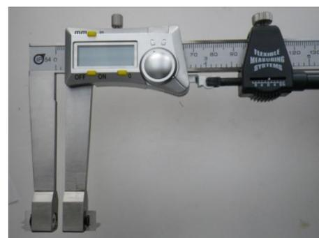
Thread inserts mounted on a caliper for internal pitch diameter measurement. Can be mounted on any standard digital caliper.
