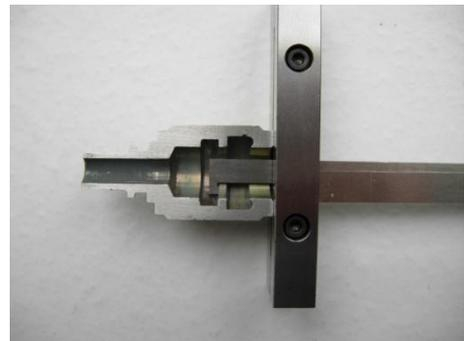
Inserts can be made to order. The ones shown below can be zeroed (0.00) at the center of the shape, thus giving the distance from the end surface to the center of the groove shape.
