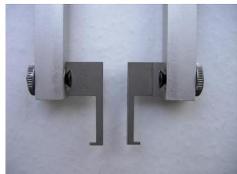
As with all internal measuring equipment a reference component is necessary. Of course, as a digital caliper is the basis then the diameter that can be measured depends on the caliper length.
